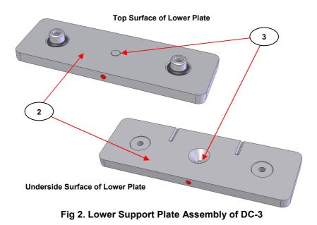
Note: There are red alignment spots on one edge of each of the upper (1) and lower (2) support plates of the DC-3 accessory. Whenever the DC-3 is constructed to bring the diamond window (3) surfaces together, the plates should always be assembled so that the red spots are together on the same side of the accessory (See Fig 3.)
